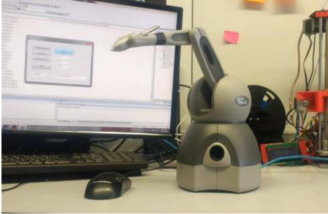
Fig. 1. Experimental platform; Geomagic touch of 3D Systems
