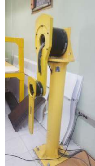
Fig. 5. 2-DOF robot manipulator used in the experiments in torque mode. That is, they act as torque sources and receive analogue voltages as a torque reference signal. Joint positions are obtained using incremental encoders which send the information to a DSP 32-bit microprocessor. The control algorithm is executed at a 2.5 millisecond sampling period on a PC-host computer.
