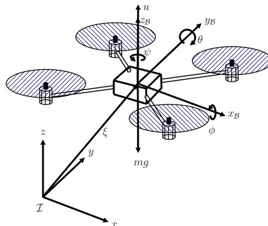
Fig. 1. Quad-rotor helicopter outline
