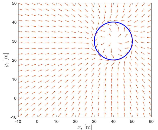
Fig. 2. Velocity field of Equation (25), with desired trajectory at position (40, 30) and radio  $r_{tr} = 10\text{m}$ .
