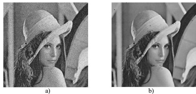
Fig. 9. Impulse noise removal. a) Salt & pepper contaminated image. b) Image with noise removed.
