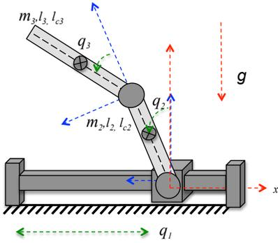
Fig. 1. Double Inverted Pendulum System (DIPCS).
