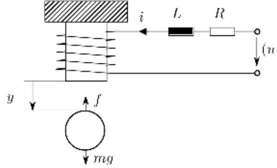
Fig. 1. Schematic diagram of the magnetic levitation system Koch et al. (2016).
