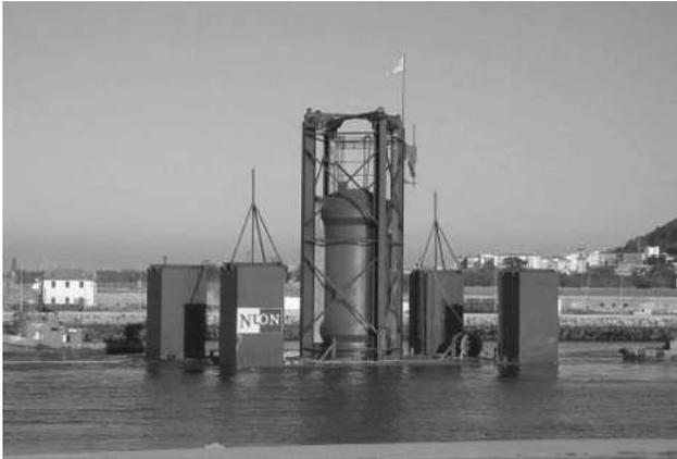
Fig. 1. The 2004 Archimedes wave swing prototype (Prado et al., 2006)
