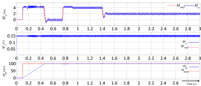
Fig. 2. Results under steady state of the C-MPC control scheme. From top: torque, flux, speed.
