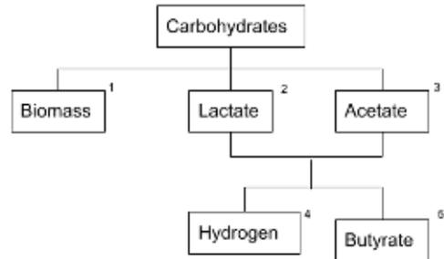
Fig. 1. Model network structure for hydrogen production via the lactate-type fermentation.
