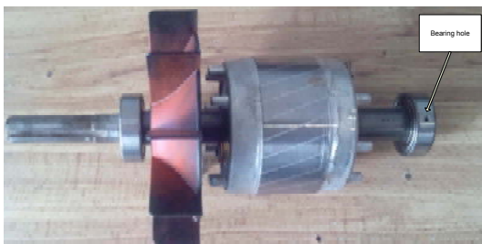
Fig. 8. Induction machine rotor shaft with a hole in the outer race bearing.
