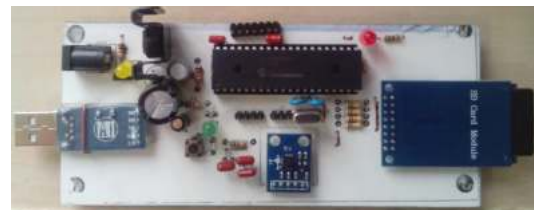
Fig. 6. Vibration data acquisition system with a high data storage capacity.
