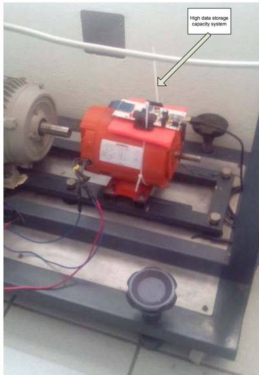
Fig. 7. The vibration data acquisition system mounted on the induction motor.
