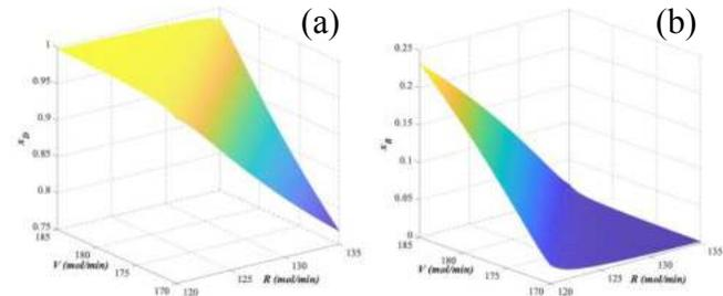
Fig. 2. Response surfaces of light component composition in the (a) distillate stream, and (b) the bottom stream
