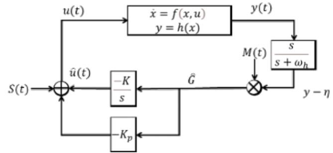
Fig. 5. Proportional-Integral perturbation-based extremum seeking scheme
