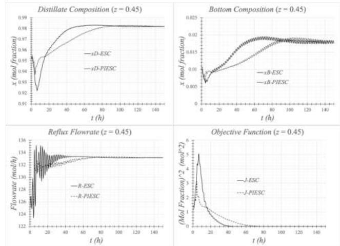
Fig. 7. Seeking of the extremum process condition for a feeding mixture of  $z = 0.45$  at  $\bar{V} = 178$  mol/h
