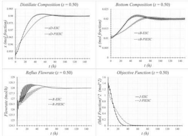
Fig. 6. Seeking of the extremum process condition for a feeding mixture of  $z = 0.50$  at  $\bar{V} = 178$  mol/h
