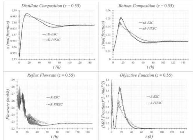
Fig. 8. Seeking of the extremum process condition for a feeding mixture of  $z = 0.55$  at  $\bar{V} = 178$  mol/h
