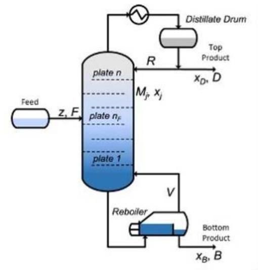
Fig. 1. Continuous distillation tray column
