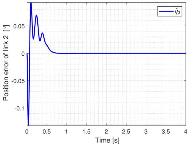
Fig. 6. Tracking error of link 2,  $\tilde{q}_2$ .
