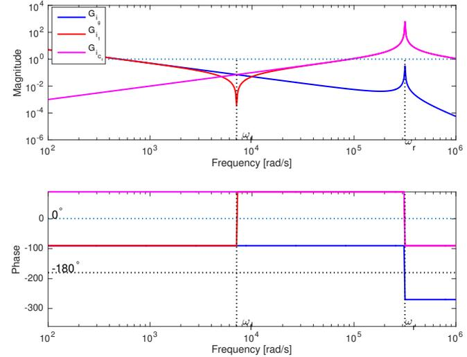
Fig. 2. Frequency responses of  $G_{i_g}(s)$  (blue graph),  $G_{i_i}(s)$  (red graph), and  $G_{i_{C_f}}(s)$  (magenta graph), where  $\omega_r$  and  $\omega_f$  are shown as dotted lines.
