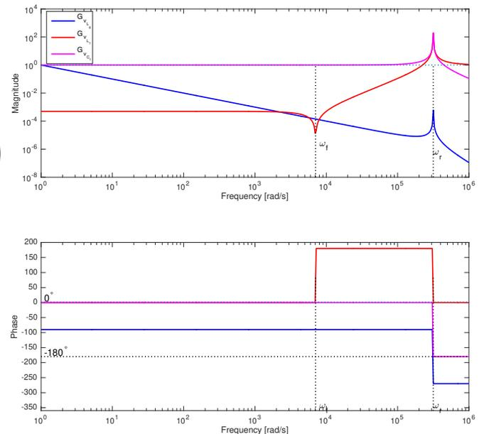
Fig. 3. Frequency responses of  $G_{v_{L_g}}(s)$  (blue graph),  $G_{v_{L_1}}(s)$  (red graph), and  $G_{v_{C_f}}(s)$  (magenta graph), where  $\omega_r$  and  $\omega_f$  are shown as dotted lines.
