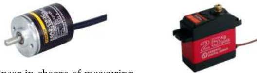
(a) Sensor in charge of measuring the angular position of the handlebars \delta . (b) Actuator to manipulate the front frame of the vehicle.
