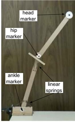
Fig. 2. Prototype built to validate the parameter estimation procedure. The stiffness at the joints was simulated using linear springs between the joints. To reduce friction, all contact surfaces were covered with teflon.
